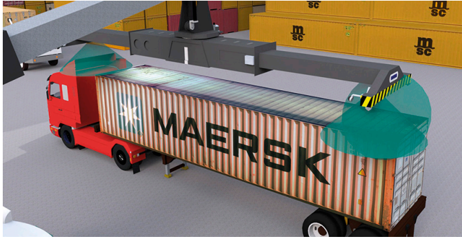
In a reach stacker system, three cameras capture images of container roof and one long side.
